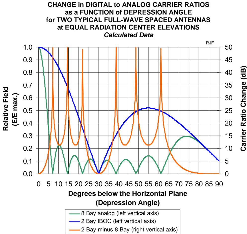
The calculated changes in carrier ratios in Figure 1 are significant: from 6dB to >50dB for some depression angles greater than about four degrees. While the nulls of installed FM antennas typically are not as deep in reality as they are in theory, their effects on the performance of FM IBOC could be an issue for highly elevated antennas, and/or where best close-in performance is required.
