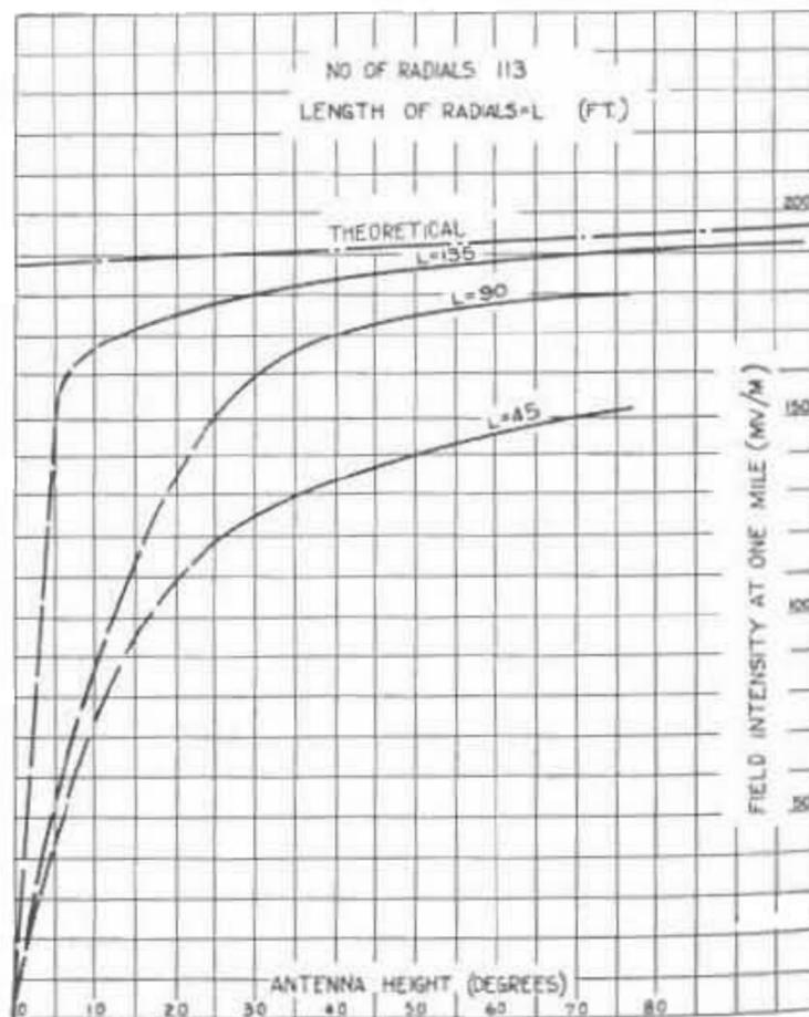
These data have been replotted in Fig. 34 in a slightly different manner. Here the number of radials is fixed at 113. The three curves of field intensity are for the three lengths of ground system tested. Fig. 35 shows similar curves when 15 radial wires are used. These two figures show the necessity of using many wires in an extended ground system. At the same time, if the ground system consists of only a few radial wires, there is no point in extending the wires to great lengths.
